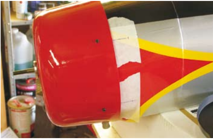
Above left ; the cowl mounting frame fits like a glove.
