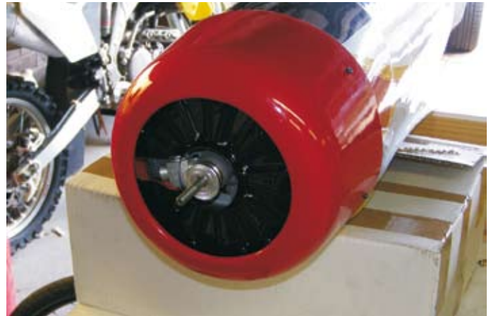
The cooling air slot is easy, cut one cylinder off the dummy radial engine.
