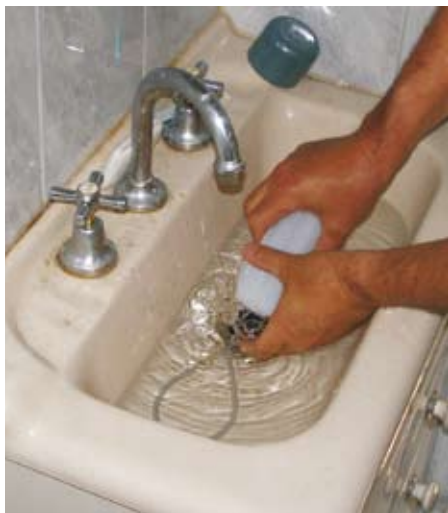
Standard tank pressure test. Pressurise the tank and if it bubbles tighten the bung half a turn each time until it stops.
