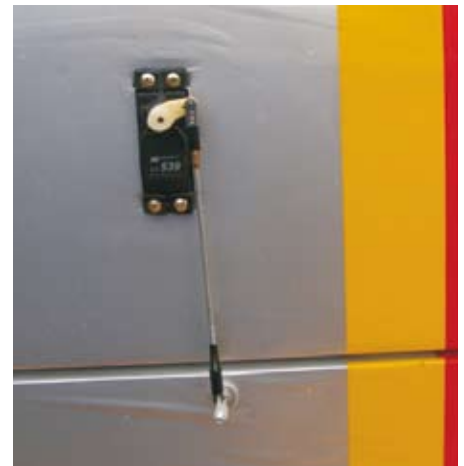
Angling the aileron servo arm forward provides mechanical differential. Don't forget the output screw.
