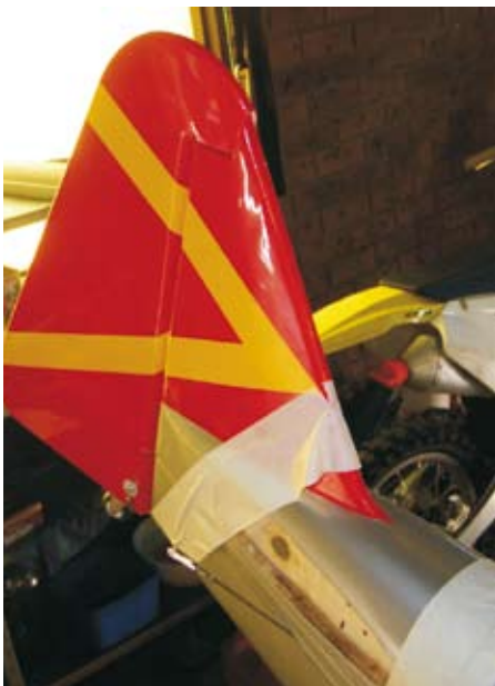
Holding the fin assembly in place until the 30 minute epoxy dries.
