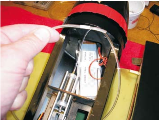
Balsawood battery box to take 4 s 3200 mAh LiPo battery pack.
