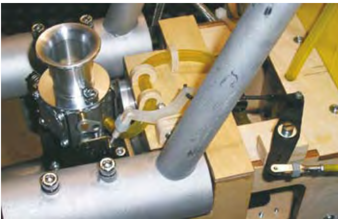
Close ups of the modified throttle linkage for a petrol engine. If using a glow motor the servo can be mounted at the firewall under the cowl. With an ignition system the servo must be mounted inside the fuselage and all radio wiring routed separately.
