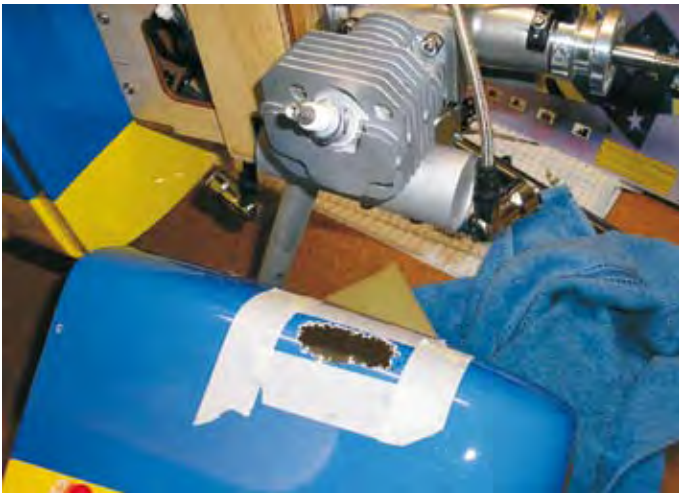
Depending on your choice of engine the cowl may need to open to clear the spark plug leads.
