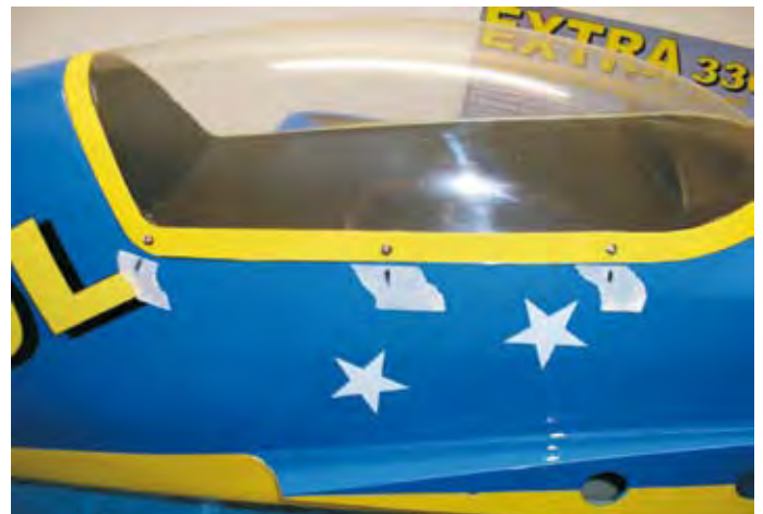
If you follow the cut lines the canopy is a perfect fit.
