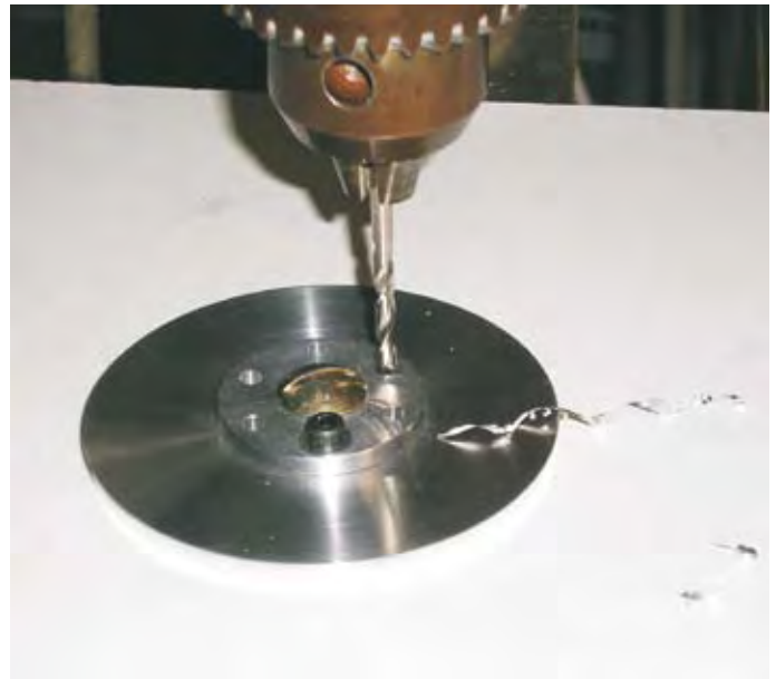
Drilling the spinner backplate.
