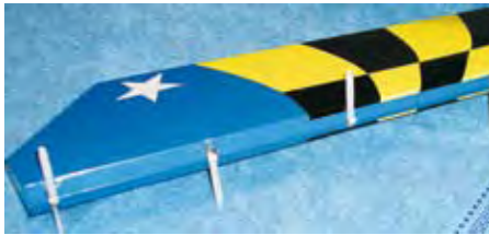
Ensure the hinge line is parallel to the hinge line is to bend them up at ninety degrees after glueing.
