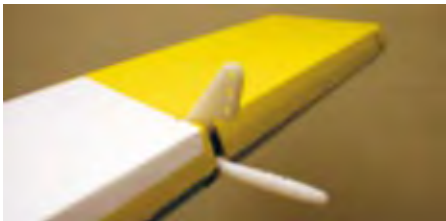
The aileron horn is integrated into a hinge point.
