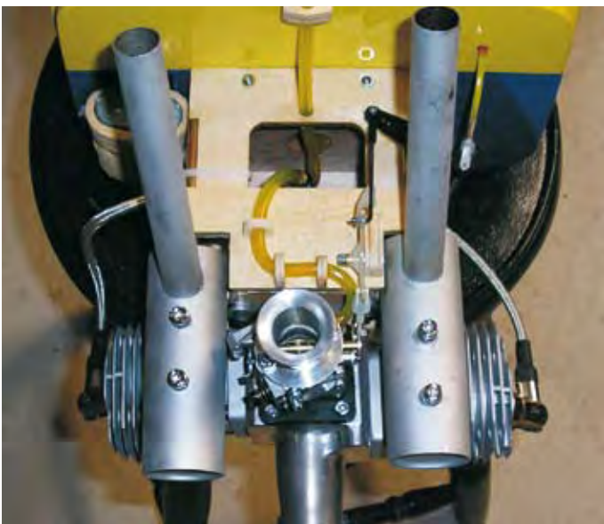
Close ups of the modified throttle linkage for a petrol engine. If using a glow motor the servo can be mounted at the firewall under the cowl. With an ignition system the servo must be mounted inside the fuselage and all radio wiring routed separately.
