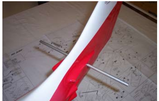
The tailplane halves are glued with epoxy.
