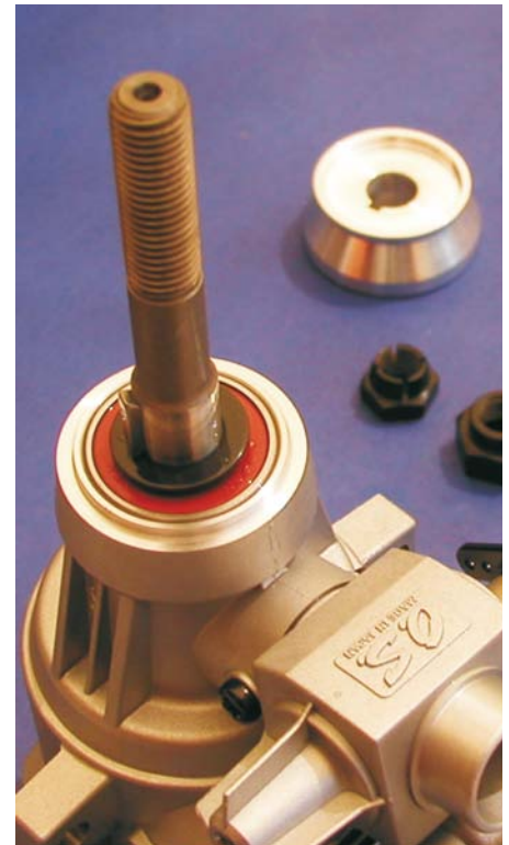
The front bearing is sealed and the prop driver is easy to remove thanks to the woodruff key.
