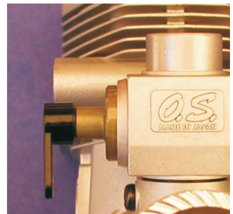
The main needle valve is angled away from the prop and the flexible extension is included. The idle need is on the same side and is easily accessible and on the other side, the throttle arm clears the crankcase.
