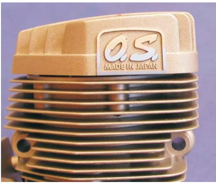
Greater cooling area at the rear of the cylinder head is good news inside an engine cowling.
