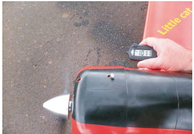
Peaked flat out at 10,110 RPM on a Bolly 15x11.
