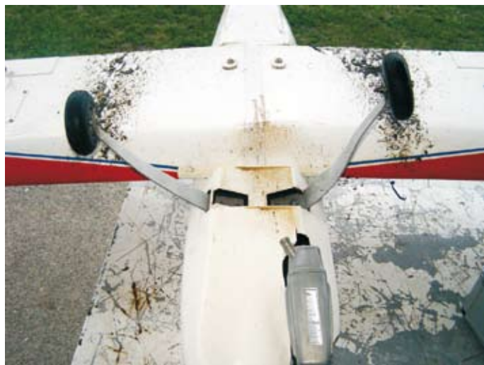
A far as maintenance of an adjustable muffler is concerned if the central screw does work loose the rear end muffler will not no longer rotate. An improvement indeed.
