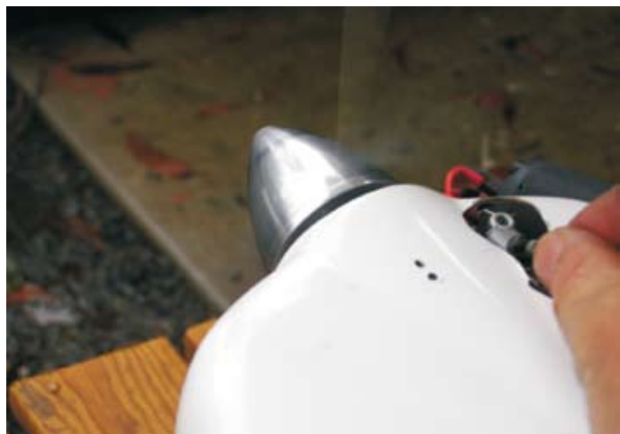
The angled needle valve makes it much safer and a lot more convenient to tune the engine.
